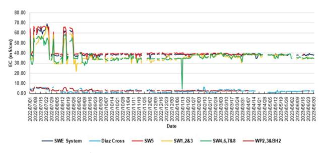
Figure 6.11: Electrical conductivity of raw water to ACRO plant
